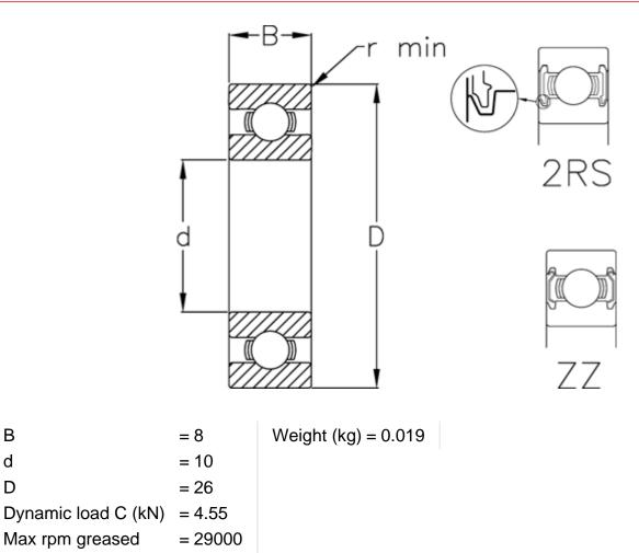
Max rpm oil lubricated = 34000 r min = 0.3
